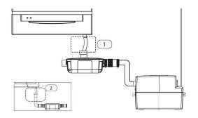
1 and 2: compulsory air intake (at inlet)
