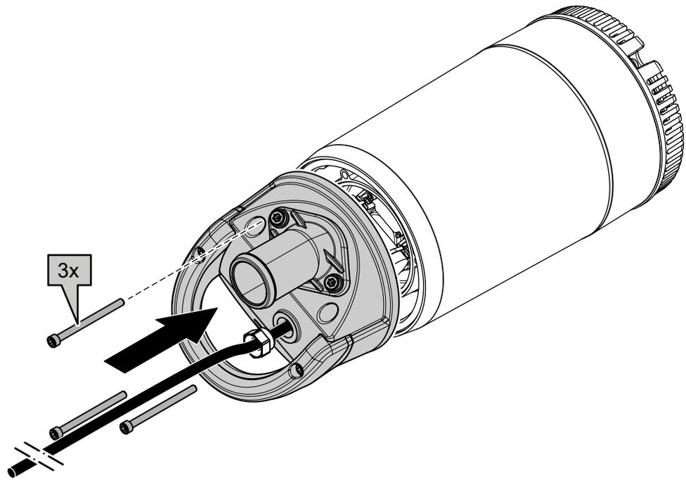
4. Tighten the cable entry.
