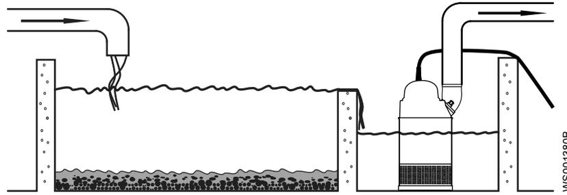
Figure 2: Settling pump-sump
