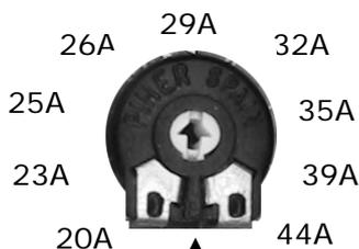
Set the current protection of the motor at a value superior of about 10-20% of the nominal current.
