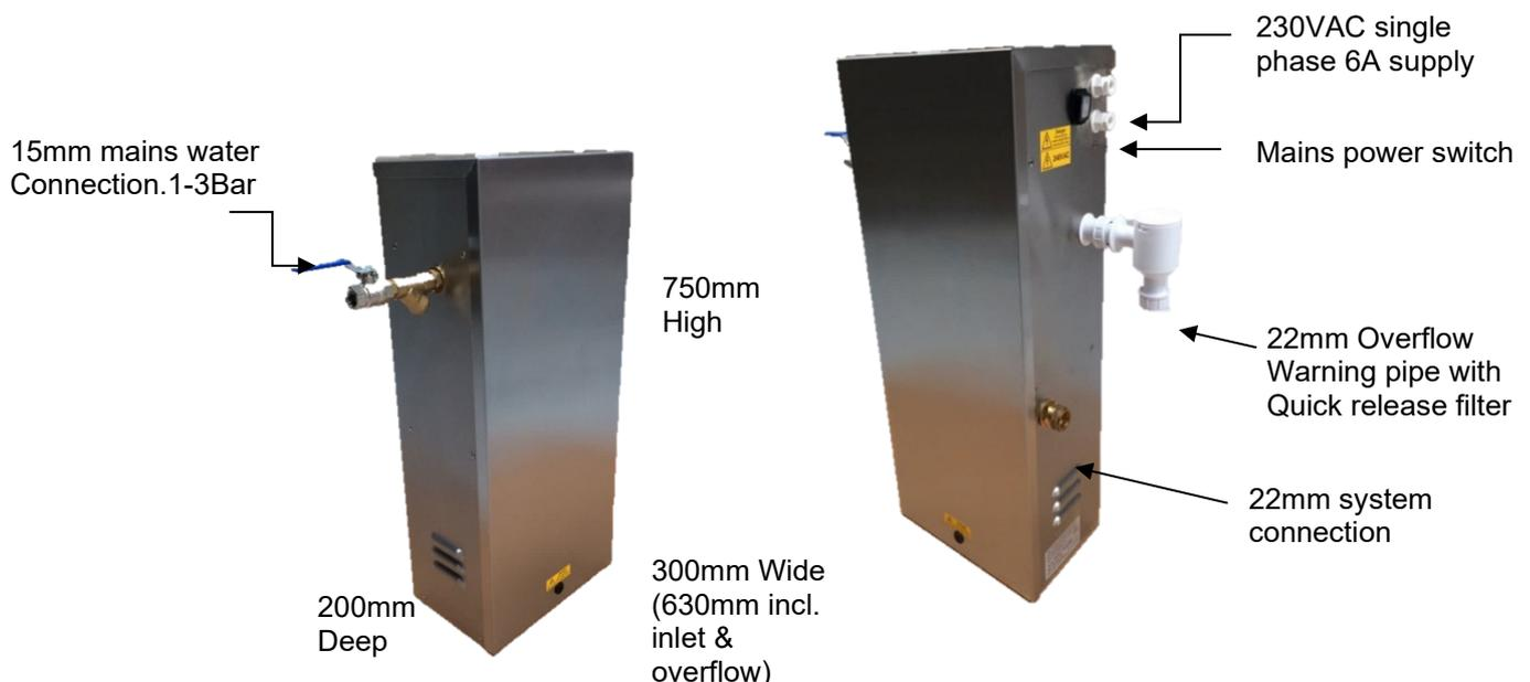
**Fig. 1.2 External Connections**
