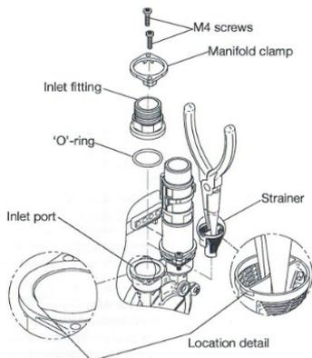
**Fig 2.1 Pump inlet filter/suction strainer**
