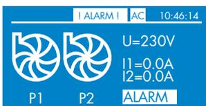
As soon as the fault disappears, return to the general screen on which an alarm notification appears. To remove the alarm notification, simply press one of the two forced-on buttons. Details of the alarms can be consulted in the alarm log.
