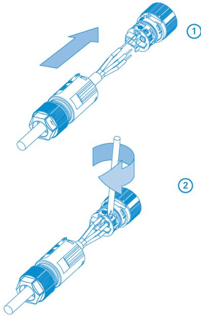
Tightening torque: 0.5 nm
