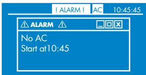
A special window giving the alarm type and the alarm time remains open.
