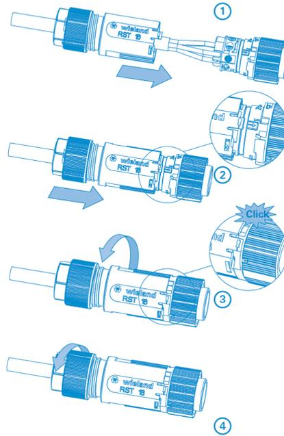
Tightening torque: 1.5 - 2 nm
