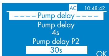
The motor activation time is pre-set to 30 seconds. After thirty seconds of continuous operation, the second motor is activated to reinforce the first one. If this parameter is too long (for the client), it is possible to change (increase or decrease) the delay.
