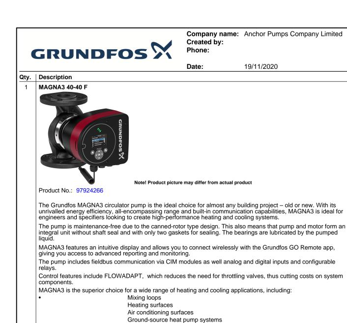
Smaller chiller applications. MAGNA3 is a single-phase pump and characterised by having the controller and control display integrated in the control box. The pump also has a built-in differential-pressure and temperature sensor.
