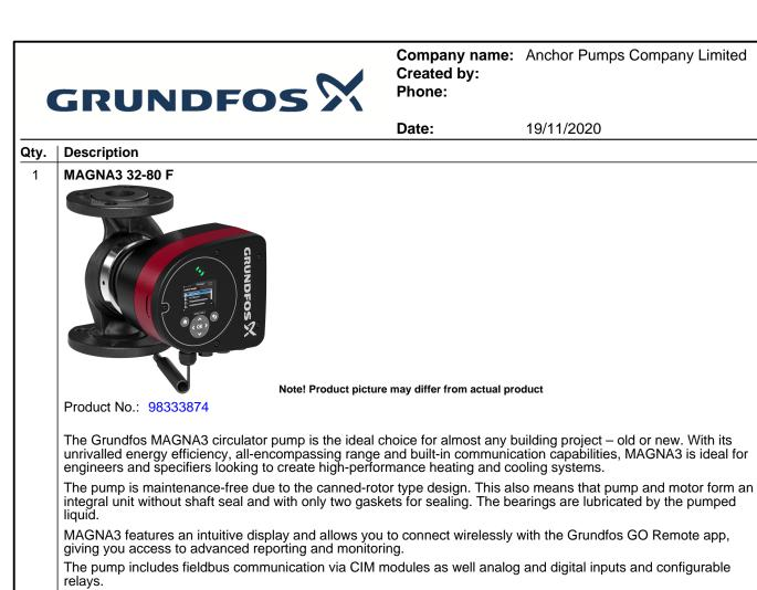
Control features include FLOWADAPT, which reduces the need for throttling valves, thus cutting costs on system components.
