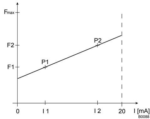
Fig. 30: Speed-current diagram for "Linear curve"
