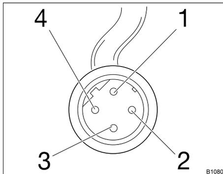
Fig. 11: Plug to "Config I/O" terminal, pin assignment
