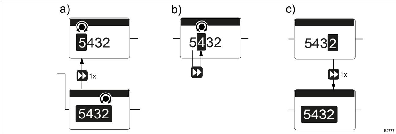
Fig. 28: a) Changing from one figure to its initial figures; b) Changing the figure; c) Returning from the last figure to the (complete) figure (to correct a wrong figure, for example).
