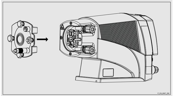
If the surfaces of the two rotor halves are perfectly flush, place bearing cover on dosing head.
