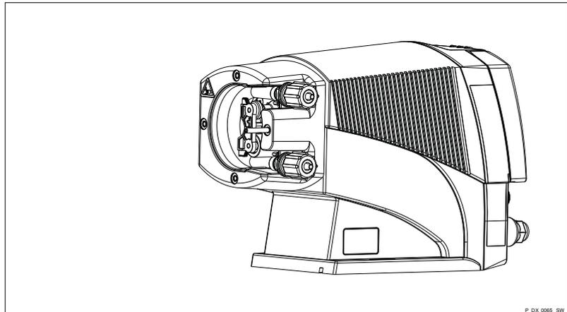
Fig. 29: Starting state of rotor (bearing cover not shown)
