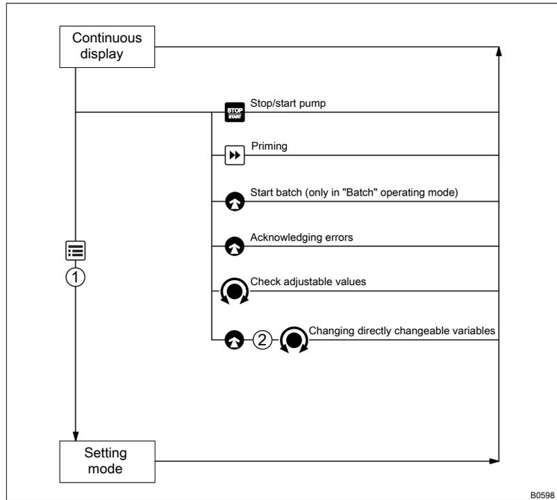
Fig. 35: Control options using keys and locking options
