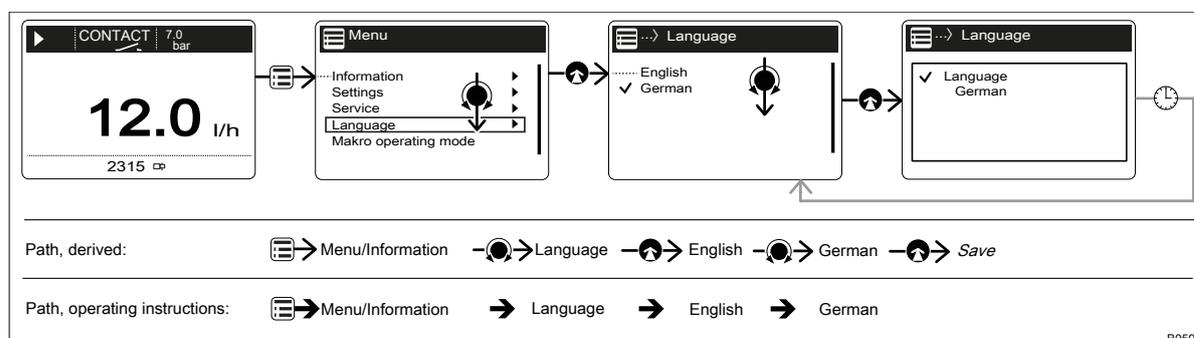
Fig. 27: "Setting up the language": As an example of set-up and path displays
