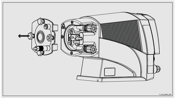
Loosen 4 star screws on dosing head and remove with bearing cover.
