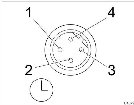
Fig. 10: "Config I/O" terminal, pin assignment
