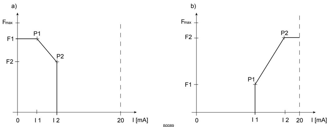
Fig. 31: Speed-current diagram for a) Lower side band, b) Upper side band
