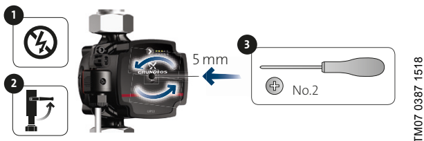
Fig. 23 Deblocking the shaft
