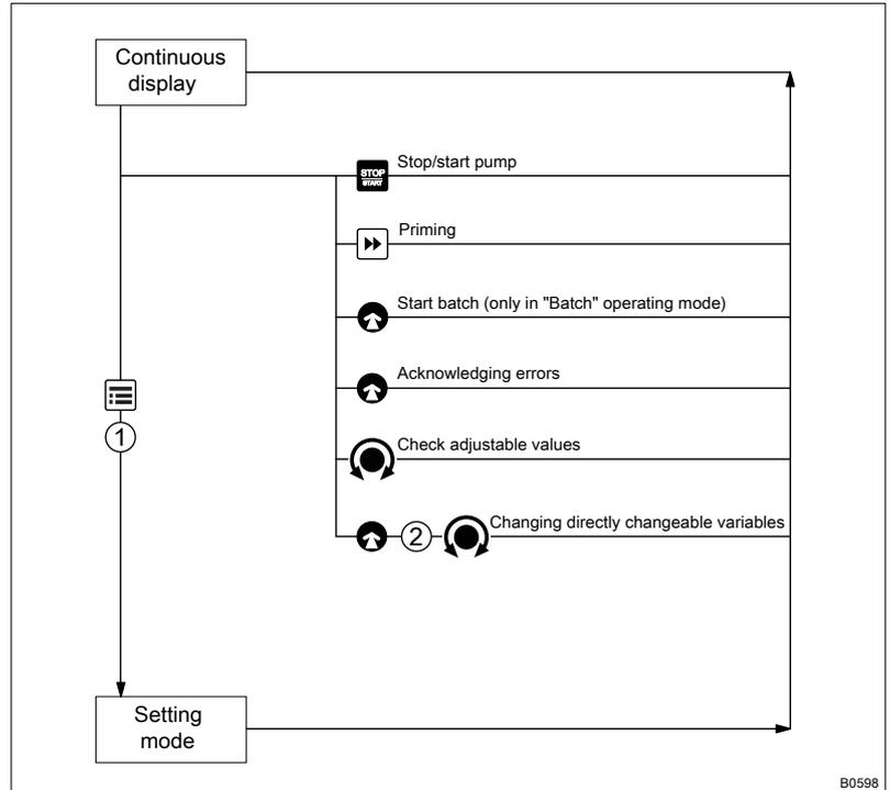
Fig. 36: Control options using keys and locking options
