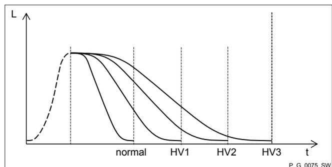
Fig. 8: Suction stroke metering profiles with stroke  $L$  and time  $t$
