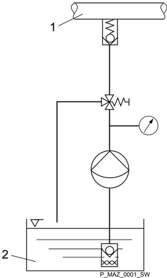
Fig. 13: Standard installation
