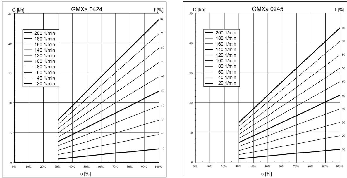
Fig. 68: Capacity C at medium back pressure depending on the stroke length s for different stroke rates f
