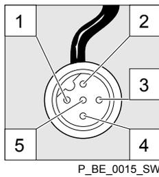
Fig. 15: Cable assignment
