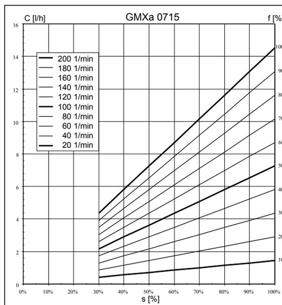
Fig. 67: Capacity  $C$  at medium back pressure depending on the stroke length  $s$  for different stroke rates  $f$
