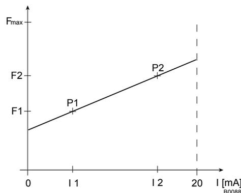
Fig. 31: Frequency-current diagram for "Linear curve"
