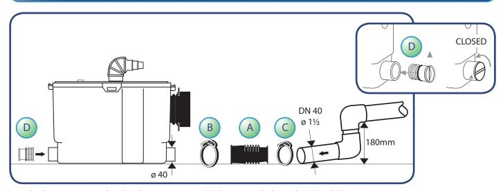
To make the connection to the side inlets, use connector (A). Secure it with plastic clips (B) and (C).
