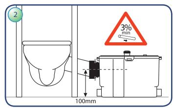
The flexible sleeve is designed to fit onto the 100mm WC pan spigot.
