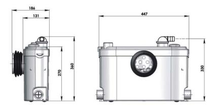
This pump/macerator has been designed to pump away the waste from a WC and the sanitary appliances in section 1.
