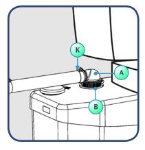
Insert the discharge elbow (A) into the rubber discharge pipe which rises up through the lid, turn to the desired direction and secure with the metal hose clip provided (32-50mm) (B). Then connect the hose to it using the 20-32mm metal hose clip (K), making sure the hose is not kinked.
