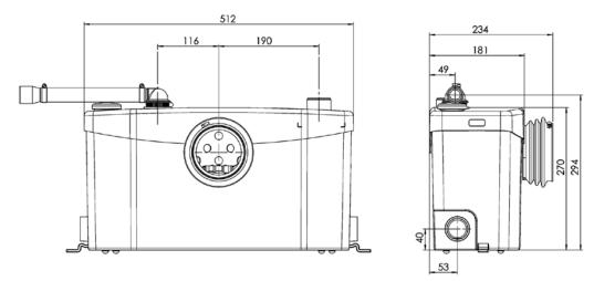
This pump/macerator has been designed to pump away the waste from a WC and the sanitary appliances in step 1.
