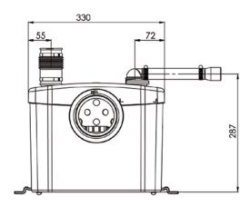
This pump/macerator has been designed to pump away the waste from a WC and the sanitary appliances in step 1.
