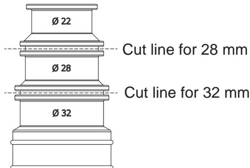
3.26 Fit the adjustable clips over the adaptor (note: fit the top one over the required pipe size section).
