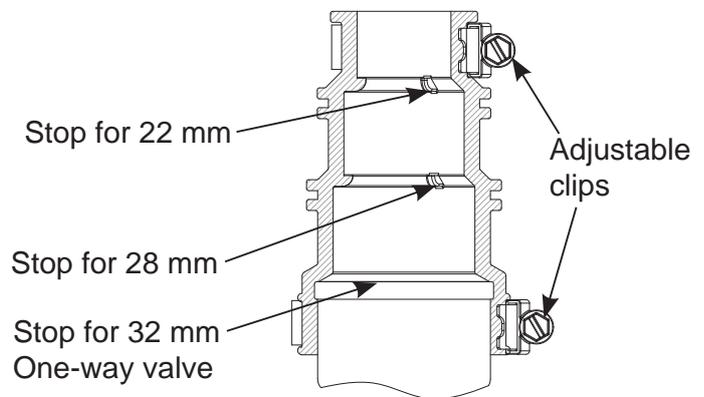
3.27 The non-return valve can then be fitted to the connector on the flexible pipe from the unit, ensuring that the rubber sealing washer is fitted, and it is tightened to produce a water tight seal.
