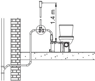
3.13 If the discharge is lower than the unit, to prevent water siphoning from the outlet pipe, an air admittance valve must be used (not supplied) capable of withstanding 6 psi, and fitted to a vertical vent pipe at least 1.4 m higher than the unit..
