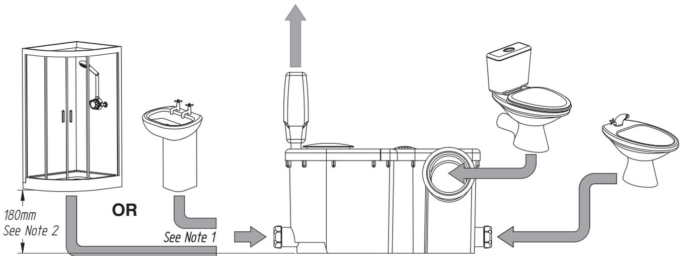
2.11 Note 1: Only connect one sanitary device per inlet connection.
