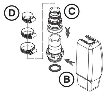
3.25 The adaptor requires cutting to fit the selected pipe size (28 or 32) as shown in the diagram below.
