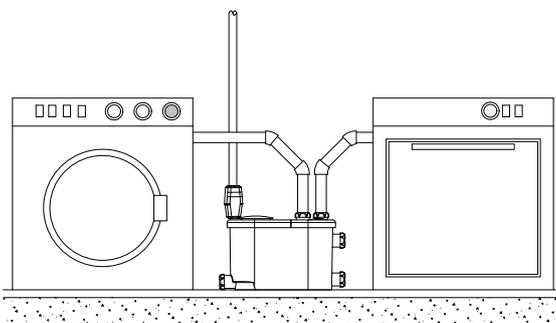
3.15 If either a dishwasher or washing machine are to be used, they must always be fitted using the top connectors.
