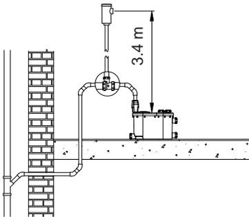
3.13 If the discharge is lower than the unit, to prevent water siphoning from the outlet pipe, an air admittance valve must be used (not supplied) capable of withstanding 6 psi, and fitted to a vertical vent pipe at least 3.4 m higher than the unit.
