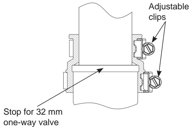
3.23 The non-return valve can then be fitted to the connector on the flexible pipe from the unit, ensuring that the rubber sealing washer is fitted, and it is tightened to produce a water tight seal.
