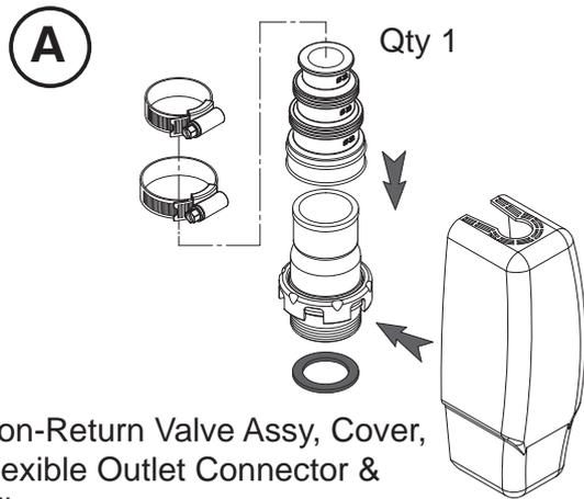
Non-Return Valve Assy, Cover, Flexible Outlet Connector & Clips
