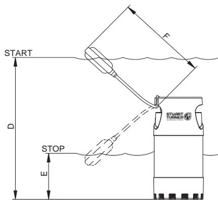
Fig. 6 Max. Float Switch Movement
