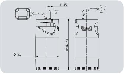
The Diver pumps are supplied complete with hose union, suitable for 25 mm (1") bore hose.
