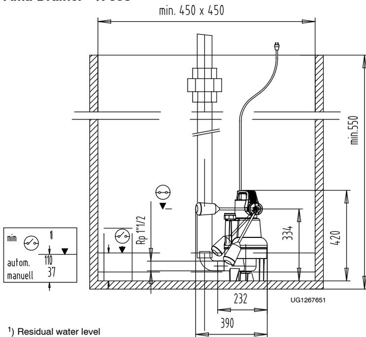
**Installation example of dual-pump station with Ama-Drainer® N 358 NE**
